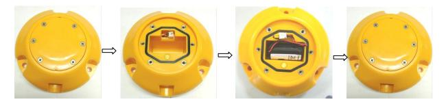
Figure 3 Battery installation or replacement
