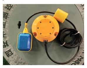
Figure 1 Manhole cover & Water level monitor
