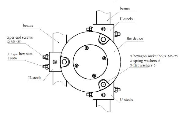
Figure 12 Installation Instruction with CS-iTWM-A02  $\,$
