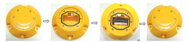
Figure 4 Battery installation or replacement
