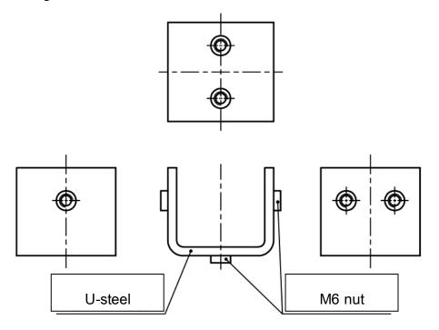
Figure 10 Installation instruction with rivet nut
