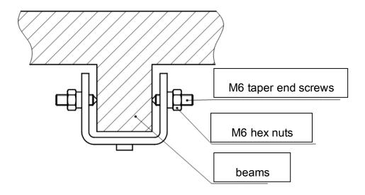
Figure 11 Installation instruction with U-steels
