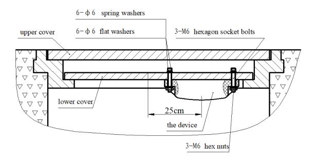
Figure 7 Installation instruction with CS-iTWM-A03
