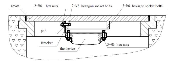
Figure 15 Installation Instruction with CS-iTWM-A01
